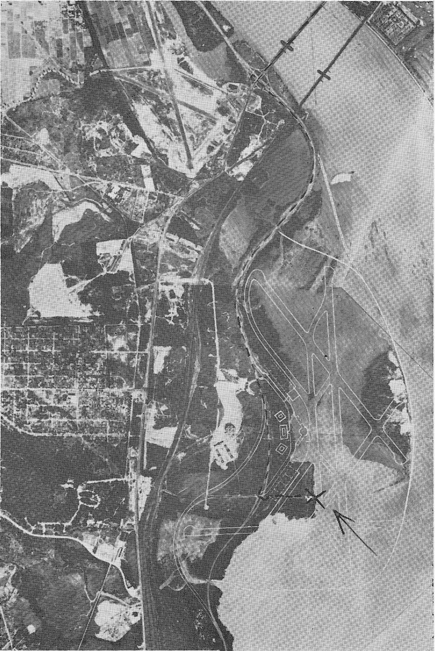
This aerial view, taken by the U.S. Coast and Geodetic Survey from 6,900 feet, shows the Hoover Airport (near the Highway Bridge) and the planned layout of the National Airport superimposed on the shore line as it existed in 1934. It also indicates the relocation of the Mt. Vernon Boulevard necessitated by the construction of the Airport. Indications of the filling operation required to build up the Airport area can be seen in the river.
