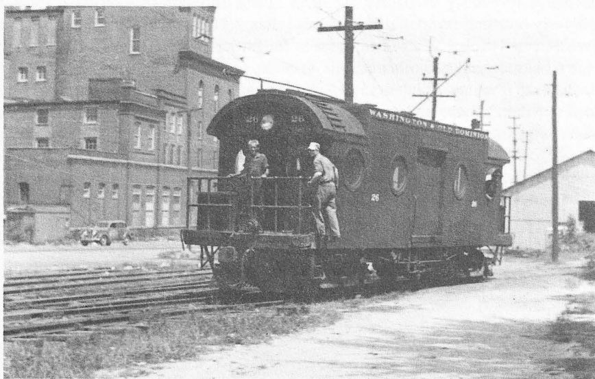
Washington & Old Dominion Railroad Box Motor Number 26, switching in Rosslyn opposite the Bottling Plant August 9, 1941. This electric freight locomotive was built in Rosslyn from wrecked passenger car components. The automobile is on Lee Highway.
